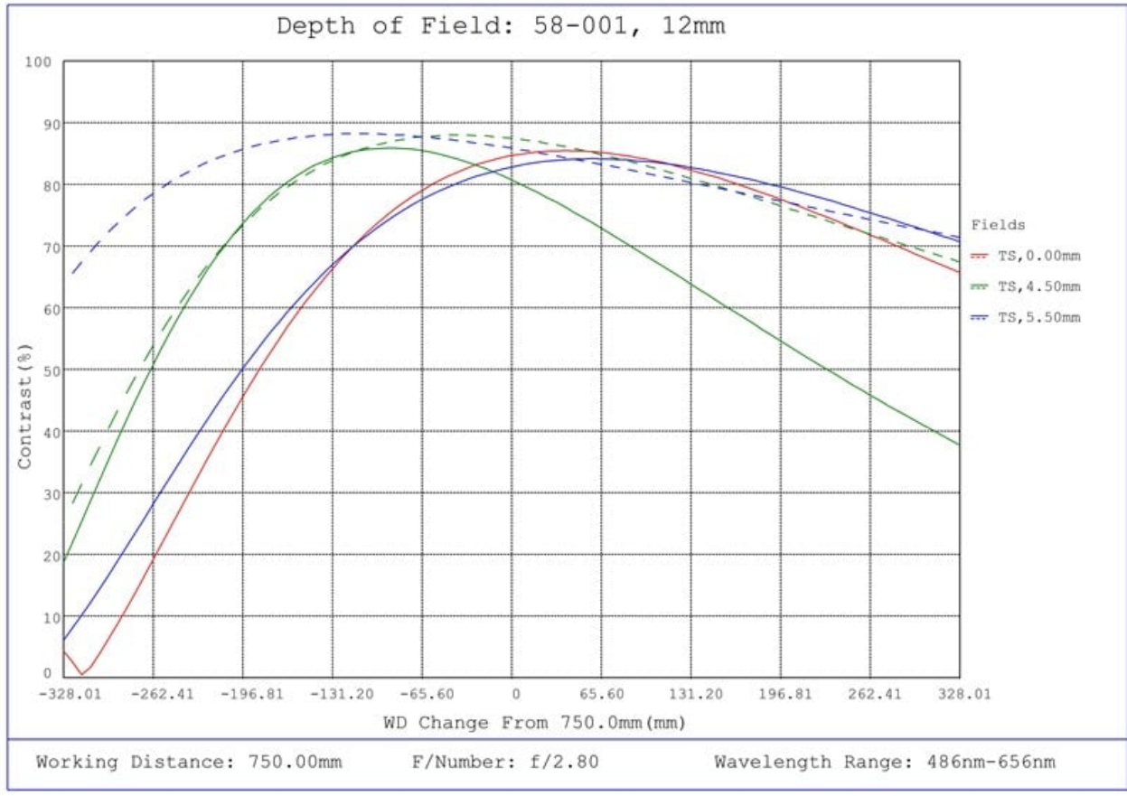
#58-001, 12mm C Series Fixed Focal Length Lens, Depth of Field Plot, 750mm Working Distance, f2.8
