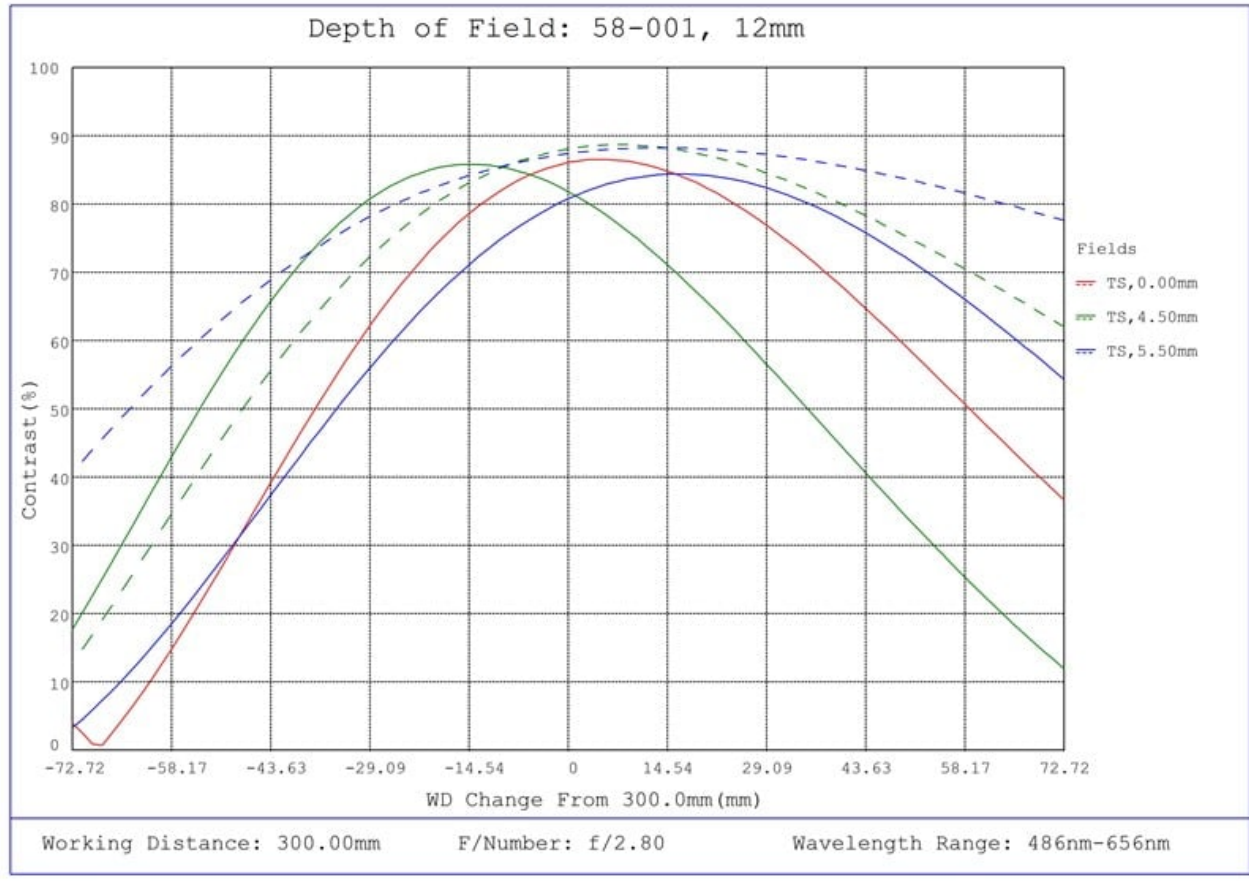
#58-001, 12mm C Series Fixed Focal Length Lens, Depth of Field Plot, 300mm Working Distance, f2.8
