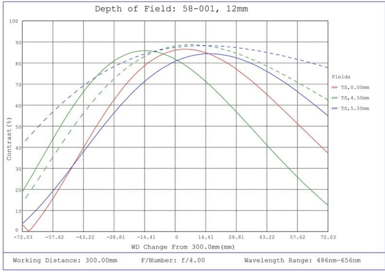
#58-001, 12mm C Series Fixed Focal Length Lens, Depth of Field Plot, 300mm Working Distance, f4
